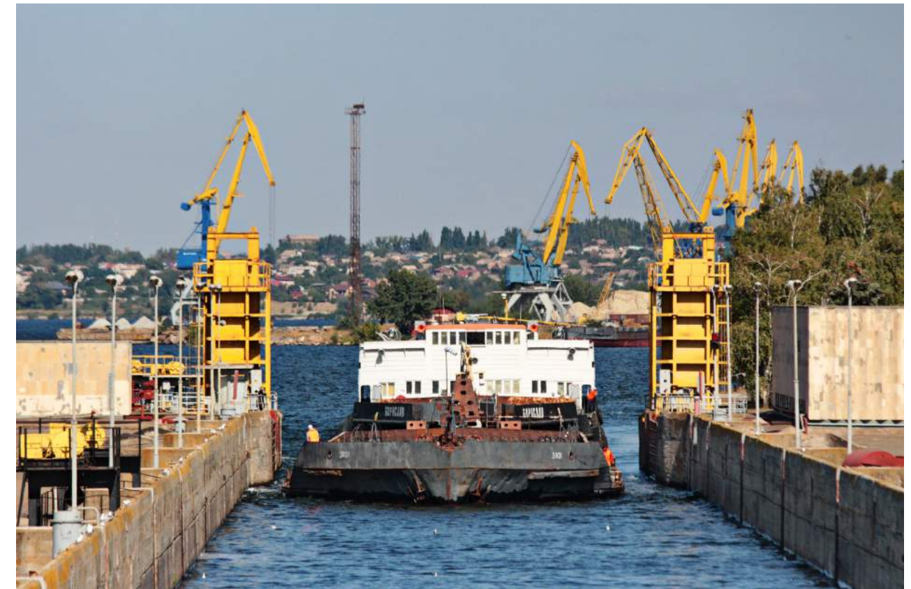
Figure 2: Photo of a barge entering the sluice in Zaporizhzhia. River port cranes seen in the background. Author: Oleksandr Malyon
