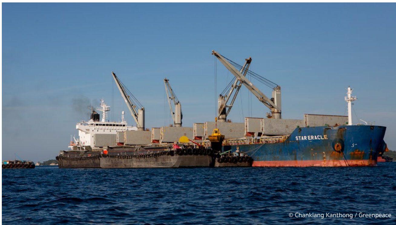
Figure 15: With the compartment doors open, a bulk carrier transfers coal using cranes and mechanical grabs onto adjacent barges at Ko Si Chang anchorage area
