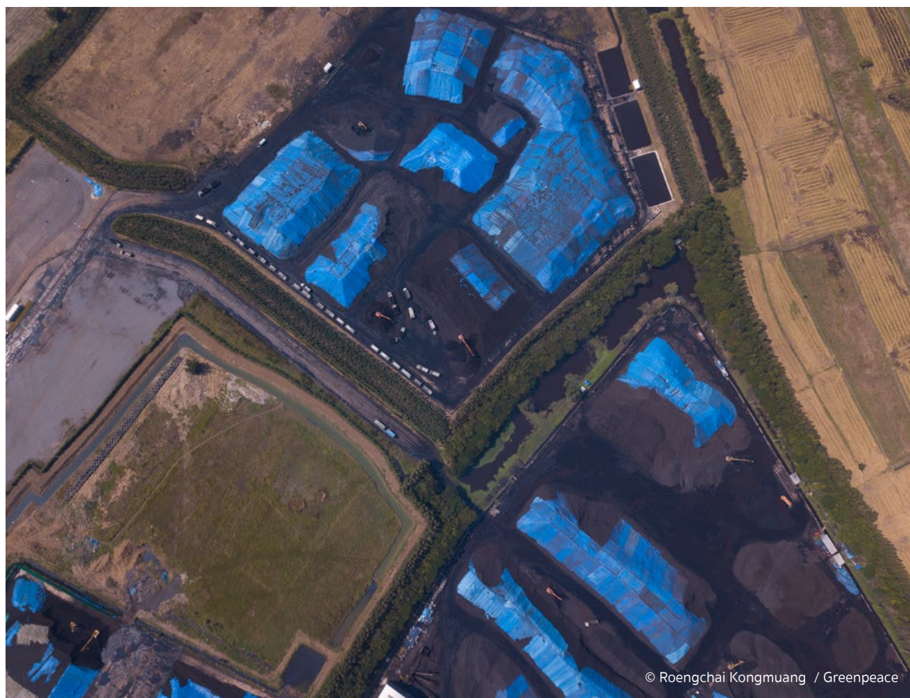
Figure 23: An aerial view over coal storage areas at Nakhon Luang District shows some part of the fuel covered by sheeting, but much left in the open air with a risk of dust dispersal
