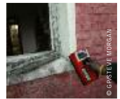
image MEASURING RADIATION LEVELS OF A HOUSE IN THE TOWN OF PRIPYAT THAT WAS LEFT ABANDONED AFTER THE CHERNOBYL NUCLEAR DISASTER, UKRAINE.
