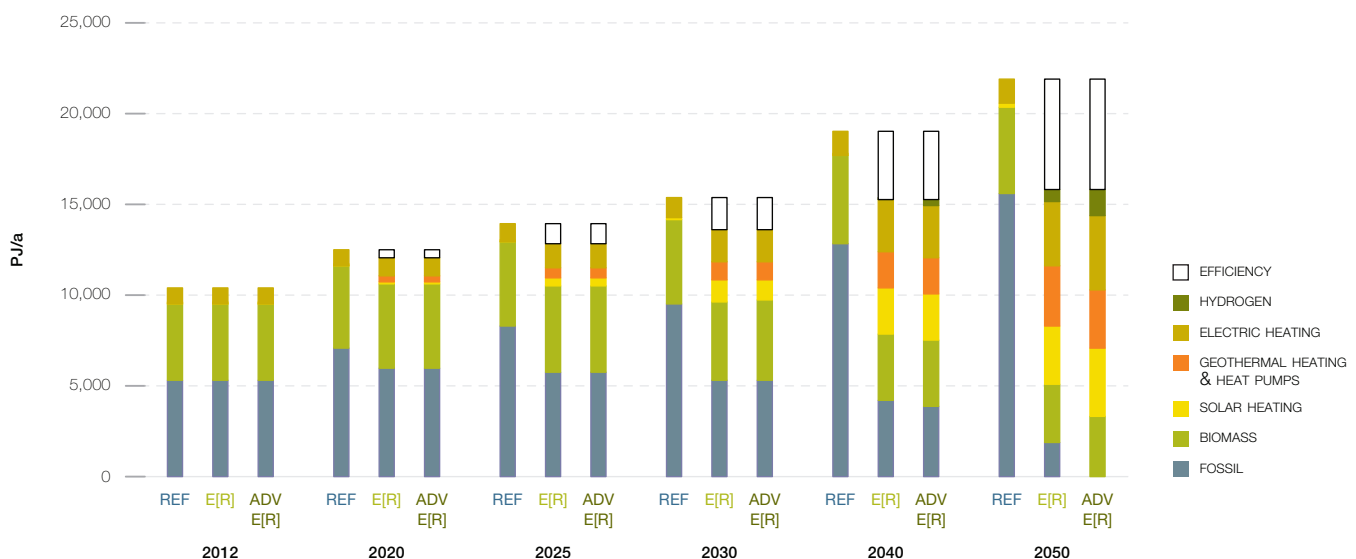
FIGURE 6.9.8 | OTHER ASIA: PROJECTION OF HEAT SUPPLY BY ENERGY CARRIER – REFERENCE, ENERGY [R]EVOLUTION, ADVANCED ENERGY [R]EVOLUTION SCENARIOS
