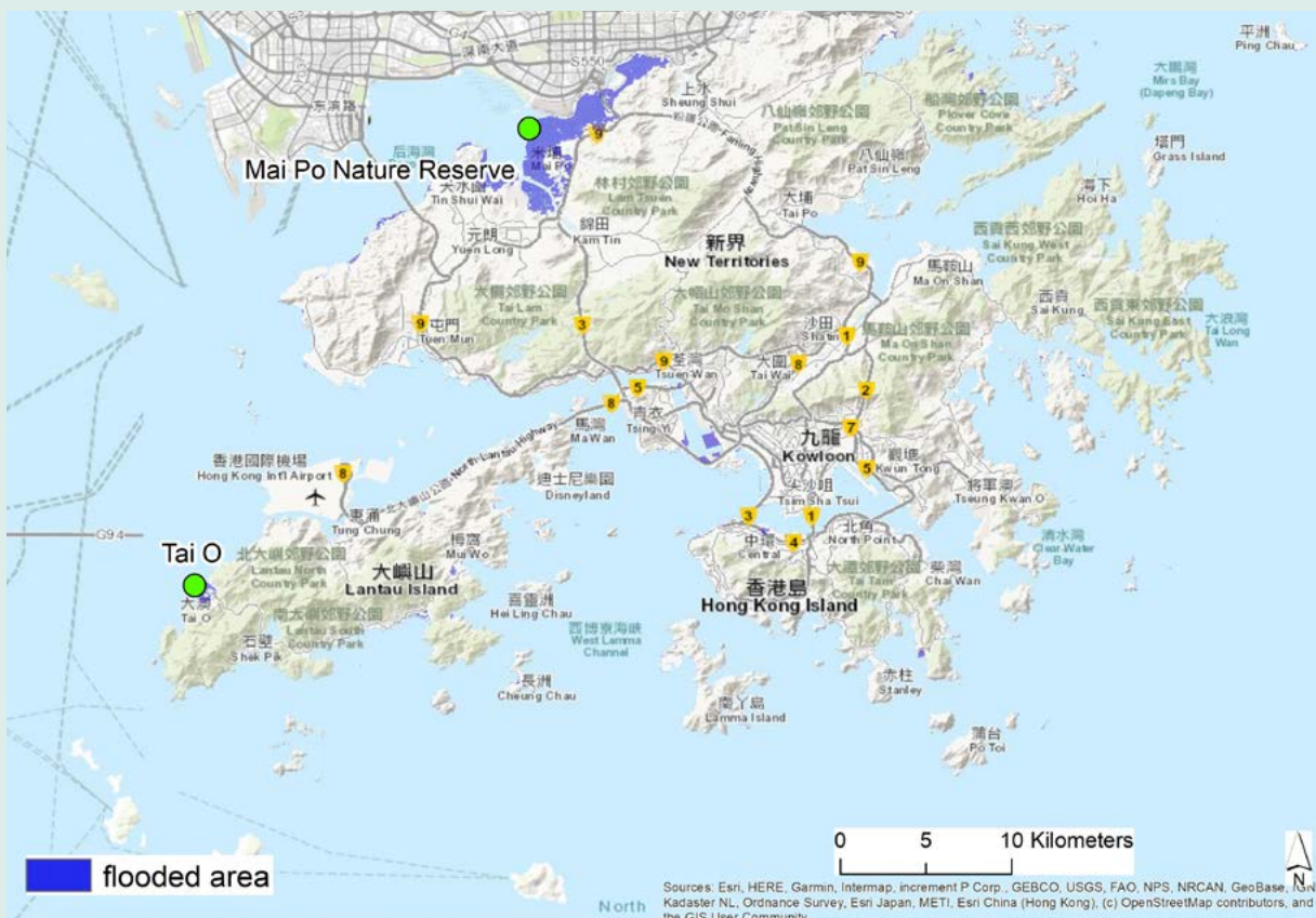
Figure 7. A geographical illustration of potential flooded areas in Hong Kong if the city experiences sea-level rise and coastal flooding in 2030, under the RCP8.5 scenario.
