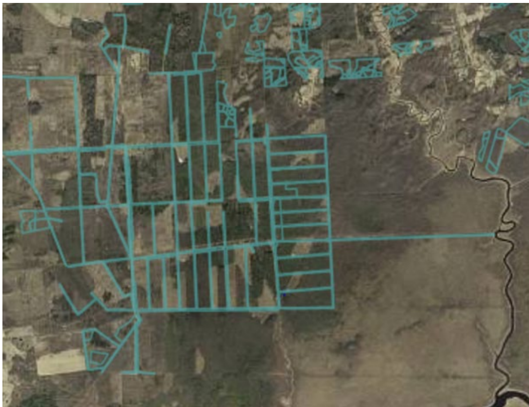
Photo 37: Satellite image of Kõrgeperve state forest with the ditches planned for renovation in light blue.
