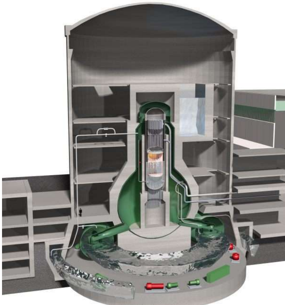
Figure 3: KKM Mark 1 Containment [Source: KUEHNI 2011]
