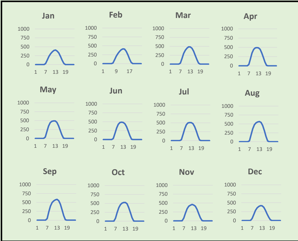
Average hourly profiles for each month Total photovoltaic power output [Wh]
