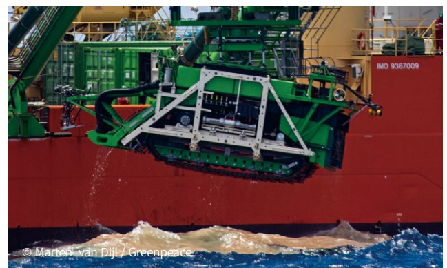
Sediment on the surface, coming from a nodule collector tested by one of the leading deep sea mining companies.
