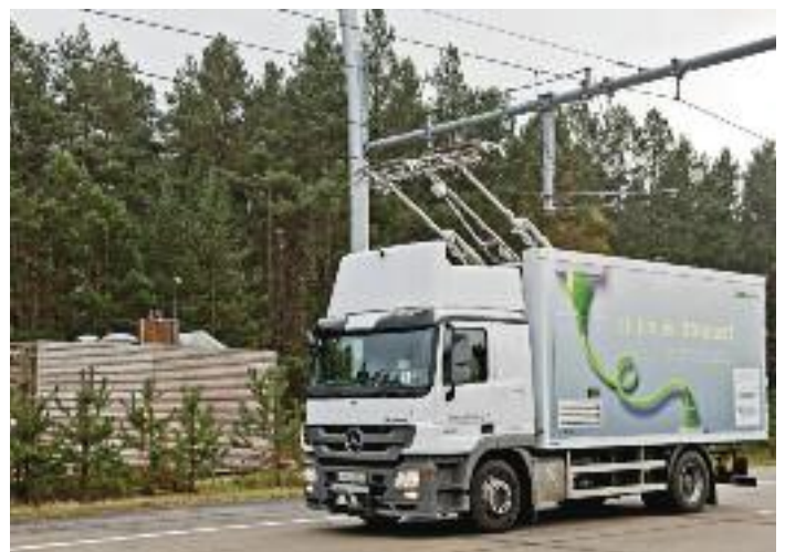
figure 9.15: HDV operating fully electrically under a catenary (picture by Siemens) 62
