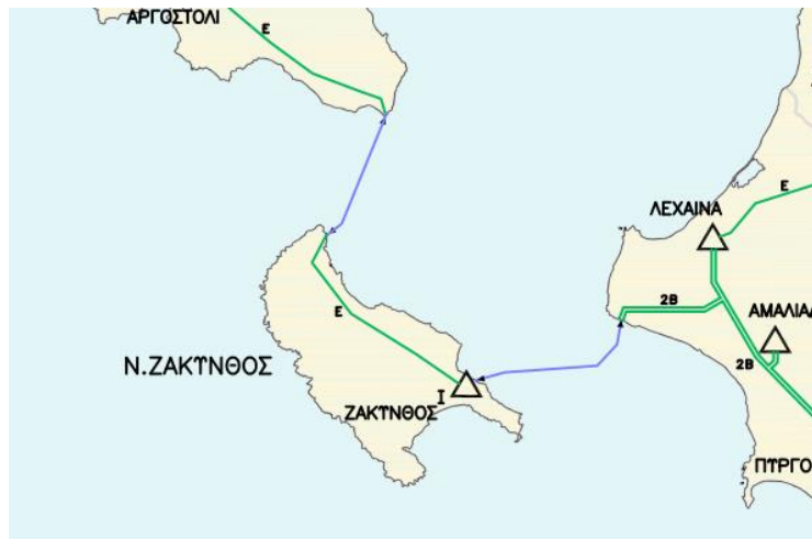
Figure 29. System of electrical infrastructure and interconnections in Zakynthos. Source: Ten-year Network Development Plan | IPTO.
