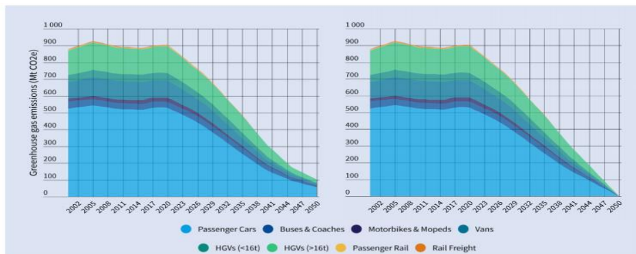
Figure 4: (Left) GHG for land transport modes with rapid adoption of ZEVs, and (Right) gradual applying ICE bans in the mid 2040s to achieve decarbonisation by 2050
