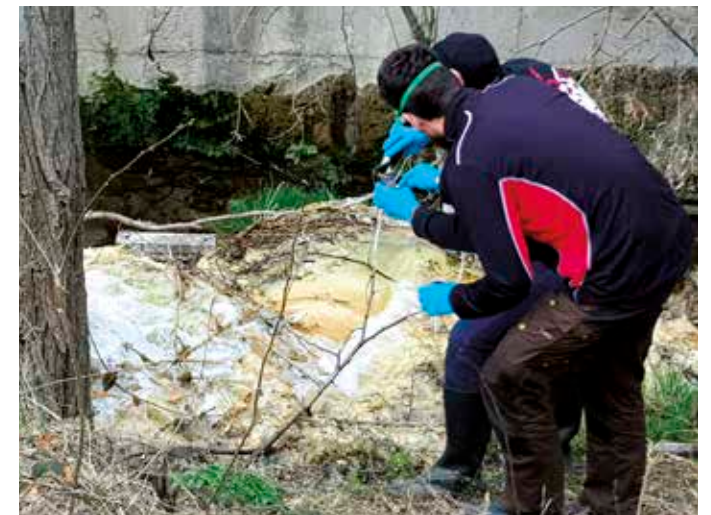
Figure 5. Collecting a sample from the sediment below the water overflowing the LEF
