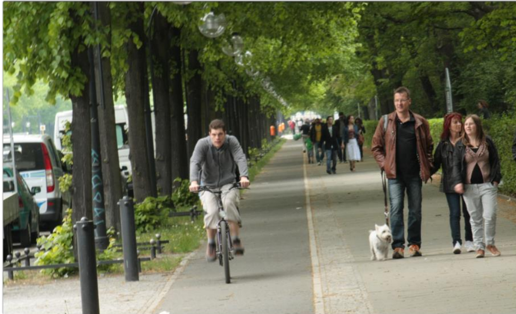
Figure 21-1 Lack of physical segregation in Berlin could lead pedestrians onto cycle paths. Source: Santhosh Kodukula
