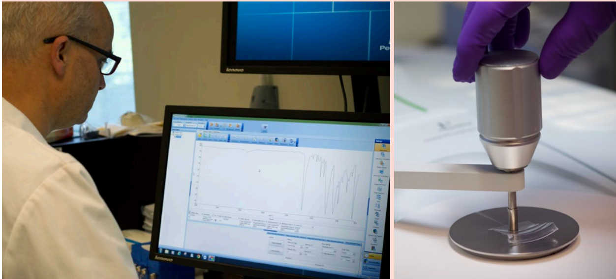
Identification of plastic and paper cup material for nine of Japan's major coffee chains through Fourier-transform infrared spectroscopy (FT-IR).
